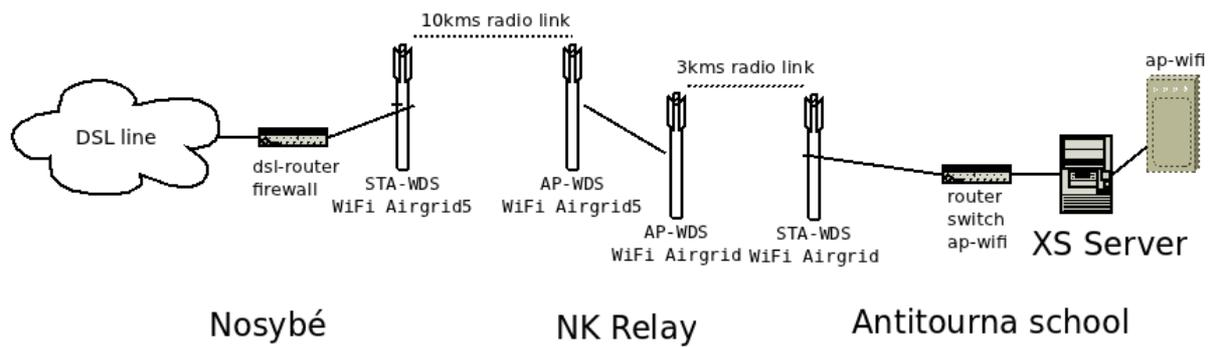
On the school, a normal Internet access architecture was configured with a switch connected to the receiving UBNT Airgrid5 and to the XS server as Internet Gateway for the local wireless network and the local services for the XOs. The XS has 2 network interfaces (one for Internet and one to the local wireless router in bridge mode to serve connectivity to the XOs)
